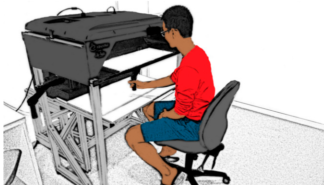
Fig. S6. Depiction of the standard setup of the KINARM device used in experiment 1 (BKIN Technologies). A similar display arrangement was used in experiments 2 and 3, although a digitizing tablet was used to collect kinematic information and participants had to volitionally move their hand back to the start position.
